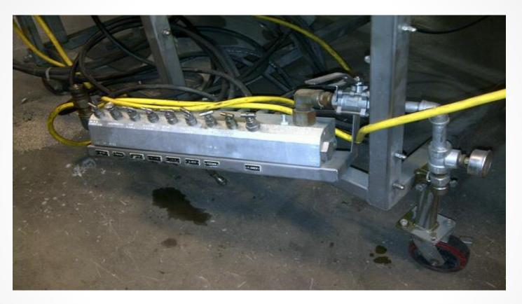
Hydraulic manifold before remanufacturing
