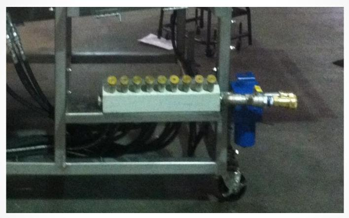
Hydraulic manifold after remanufacturing
