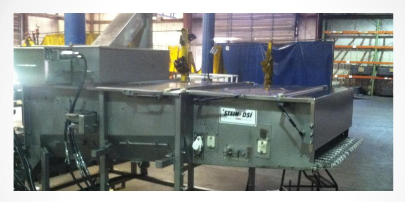
If hoods and guards are damaged or missing we make all new ones and electro-polish them before installation for a more sanitary finish
