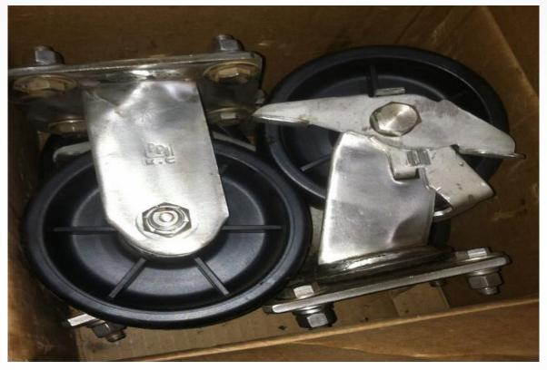
All machines come with a new set of stainless steel casters with brakes
