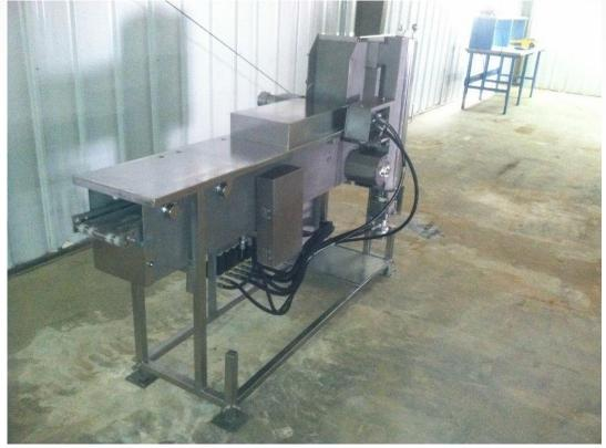
• If hoods and guards are damaged or missing we make all new ones and electro-polish them before installation for a more sanitary finish
