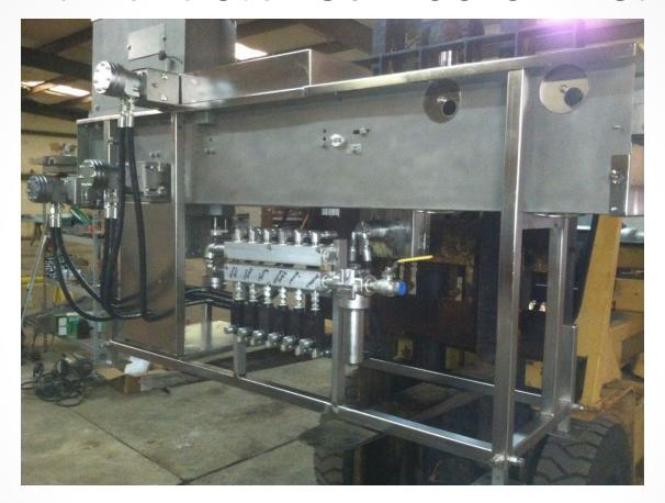
Hydraulic manifold after remanufacturing
